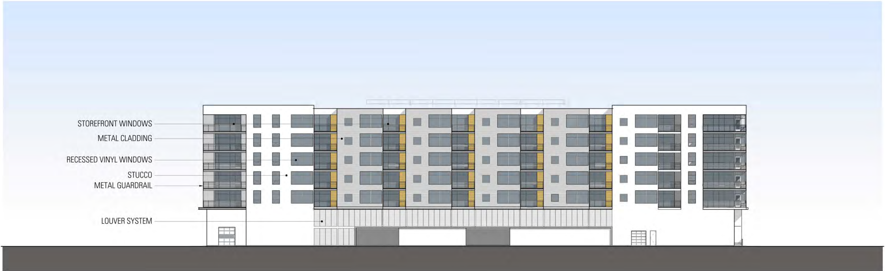
EXTERIOR ELEVATION - NORTH 1/16" = 1'-0"
