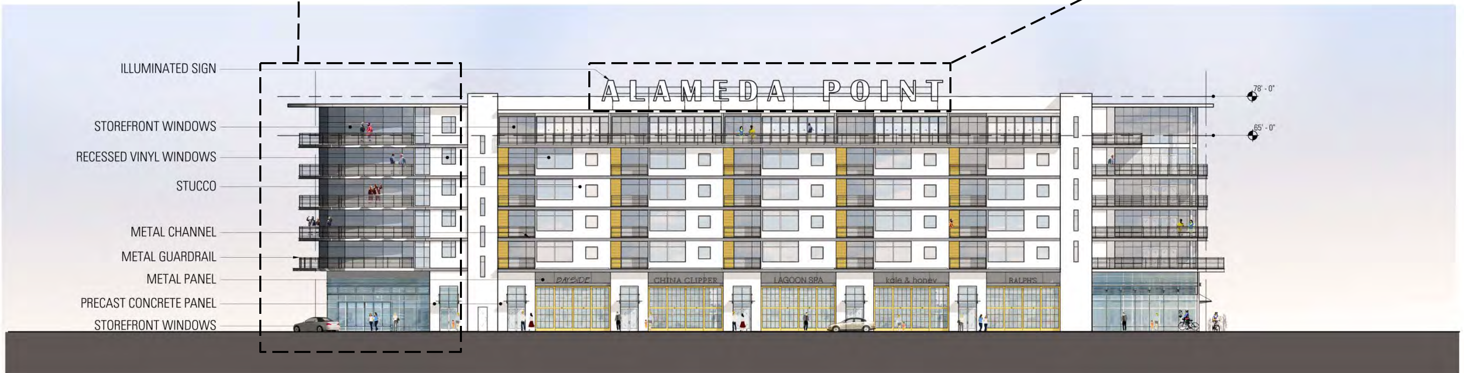
EXTERIOR ELEVATION - SOUTH 1/16" = 1'-0"
